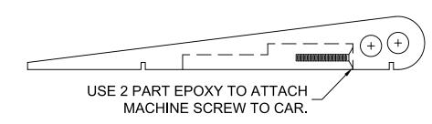
FILL THE TWO 3/8 HOLES WITH MELTED LEAD (LEAD IS POISONOUS!)
